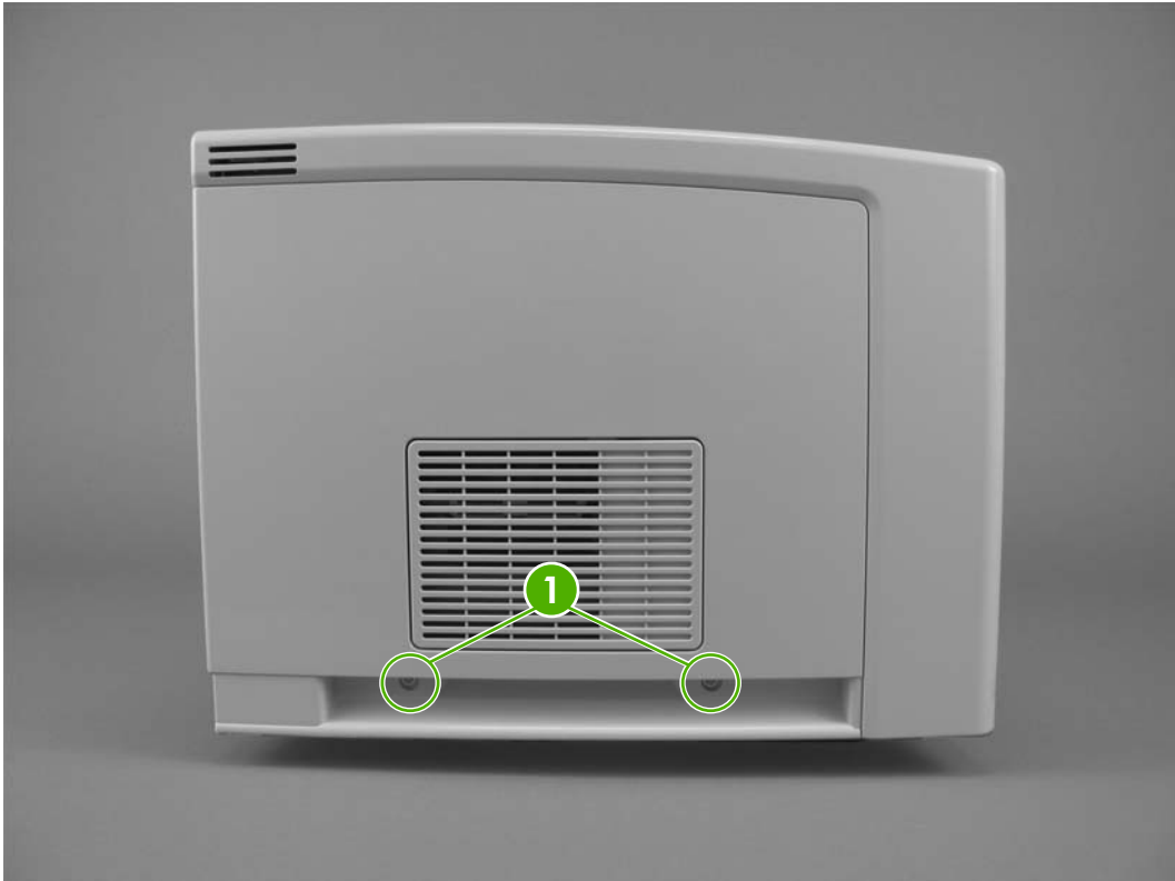
Figure 5-3 Removing the left-side cover (1 of 2)
