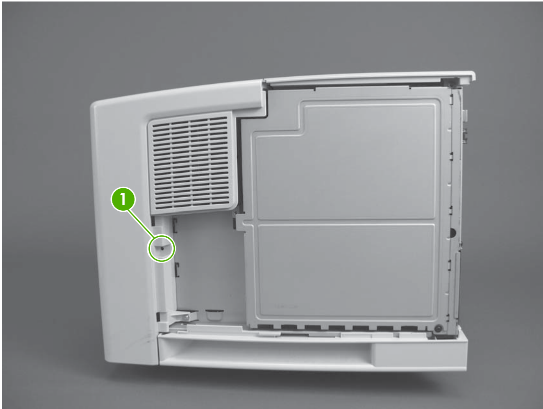
Figure 6-3 Locating the engine-test-page switch
