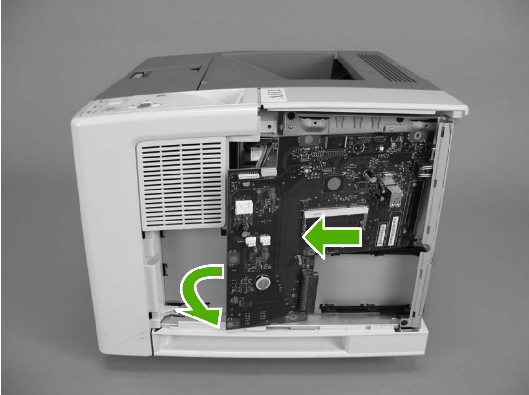
Figure 5-15 Removing the formatter (3 of 3)
