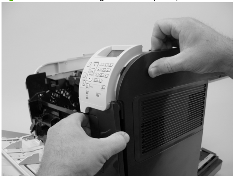
Figure 6-43 Remove the right-side cover (2 of 3)
