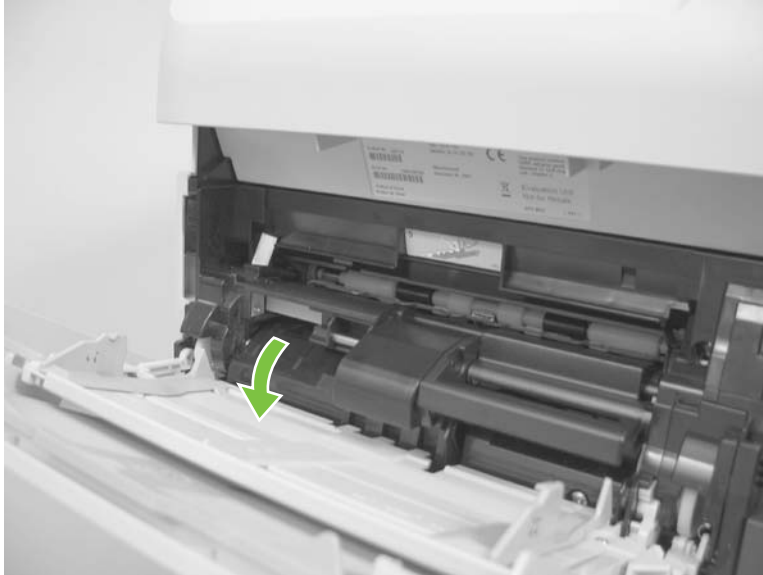
Figure 6-31 Remove the Tray 1 separation roller (1 of 3)
