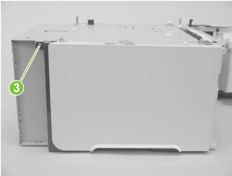
Figure 6-137 Remove the 1,500-sheet feeder left-side cover (4 of 5)
