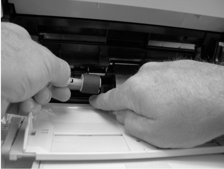
Figure 6-33 Remove the Tray 1 separation roller (3 of 3)
