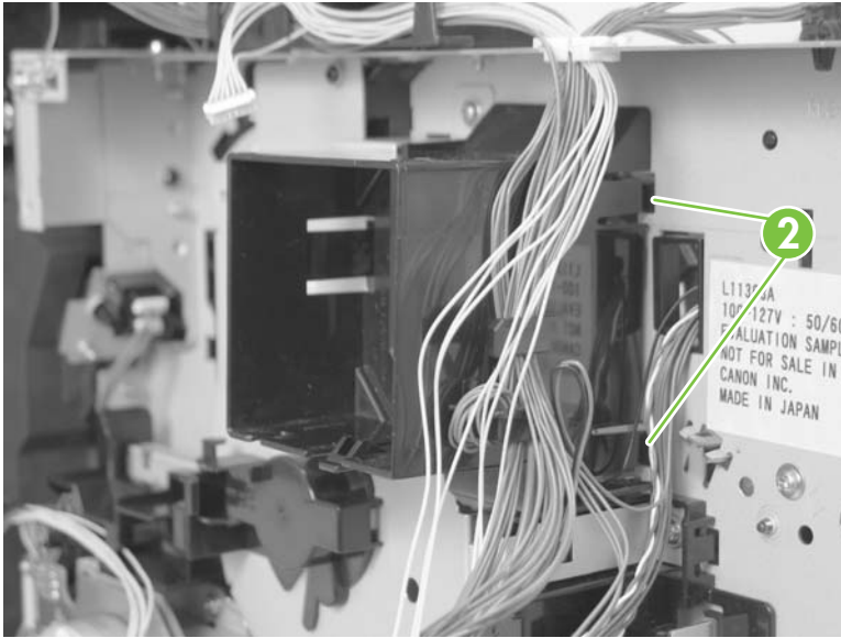
Figure 6-91 Remove the drum-drive assembly (2 of 4)
