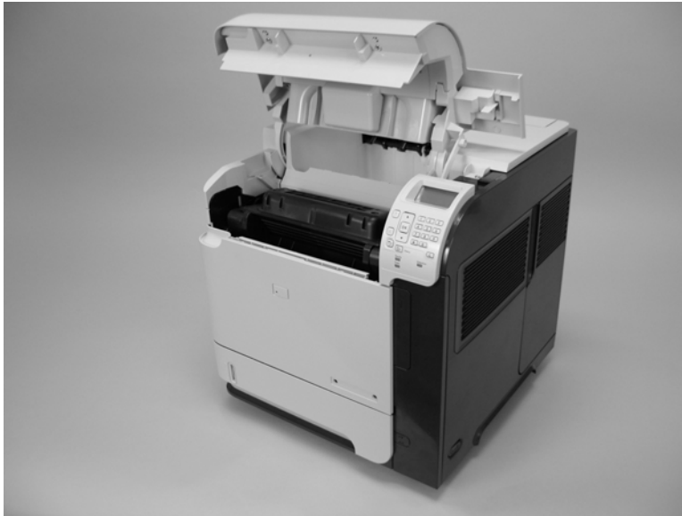
Figure 6-5 Remove the print cartridge (1 of 2)
