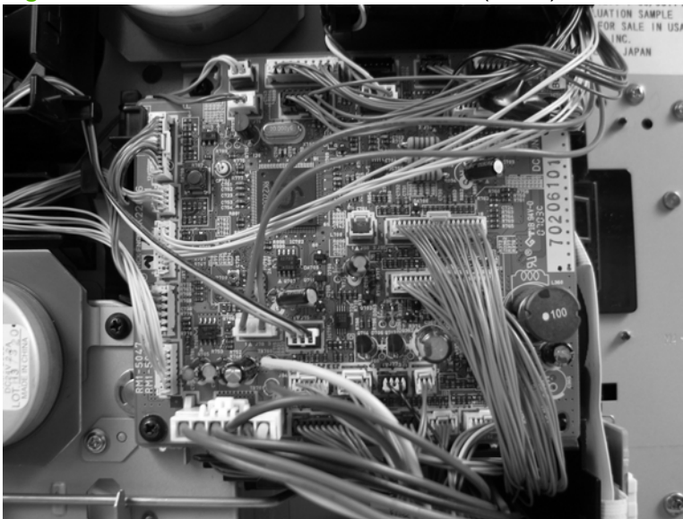
Figure 6-76 Remove the DC controller PCA (1 of 4)
